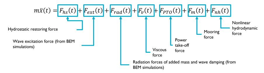
Excitation and radiation forces are determined from hydrodynamic coefficients calculated from Boundary Element Method (BEM)
